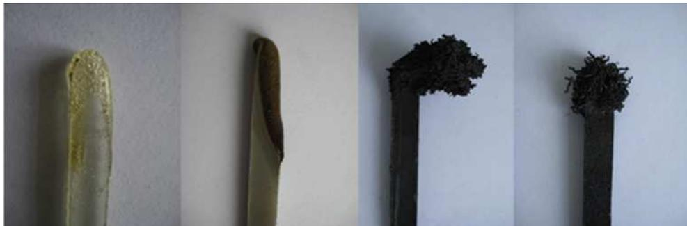
Figure 9: Photographs of PLA specimens after limiting oxygen index tests
